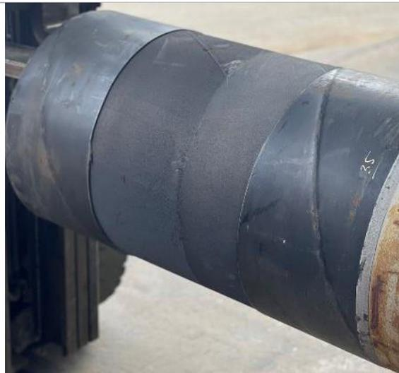
Following removal of Sintakote, all residue must be removed from steel during surface preparation.
