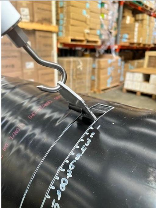
Peel Test set out in accordance with Appendix B of AS 4822;2018. Pass level is 5 kg.f (50 N) for a 25mm wide test sample.
