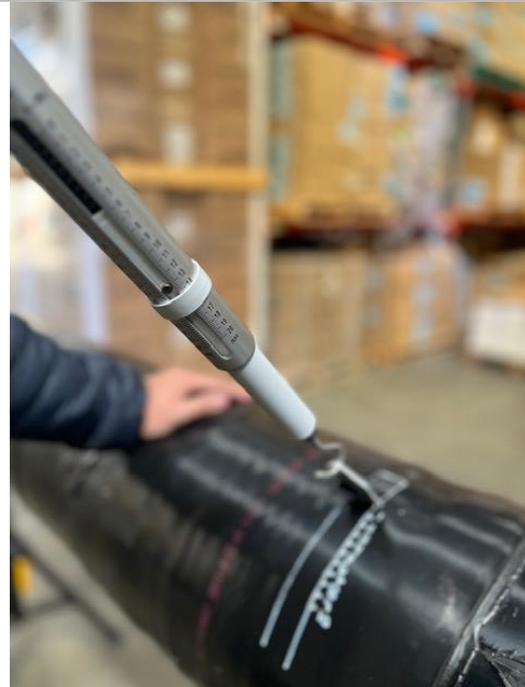
Peel Test being performed with spring gauge and custom clip in accordance with AS4822;2018.
