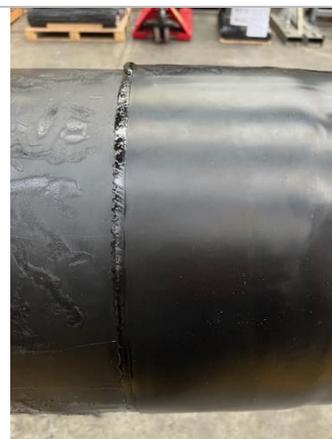
Finished sleeve with adhesive oozing from both edges of sleeve.
