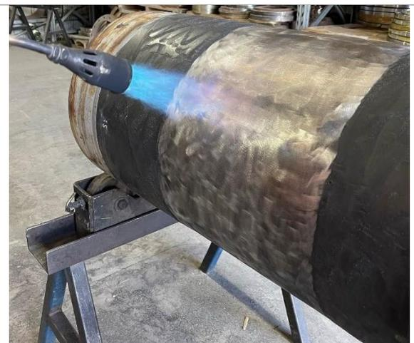
Pre-heat steel to 25°C or 3°C above dew point using the UCC KLON 114KW Gas Torch Kit
