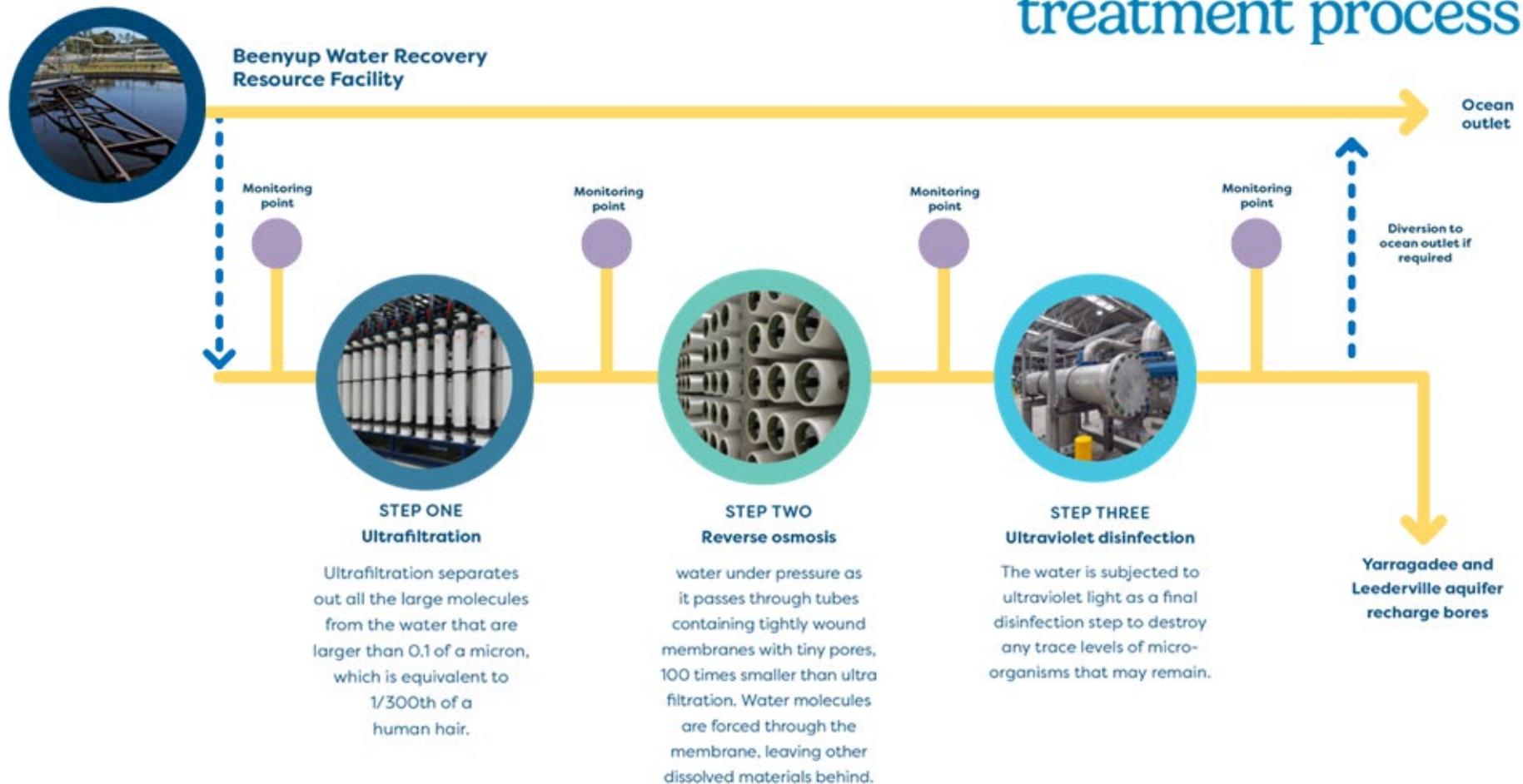
Figure 25: Advanced water treatment process
