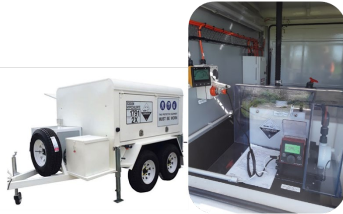
Figure 32: Mobile chlorine dosing unit
