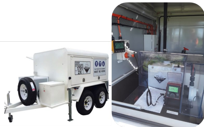
Figure 32: Mobile chlorine dosing unit
