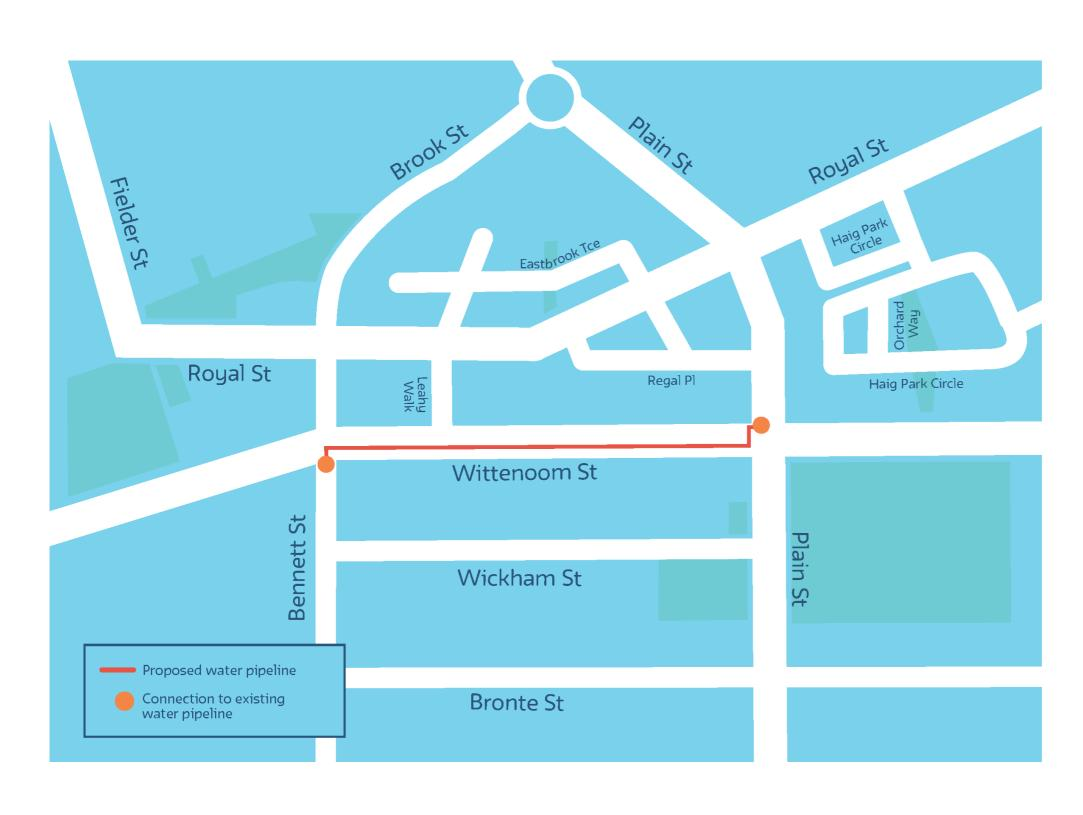
Water Corporation proposes to construct 340m of 400mm diameter below ground water main.
