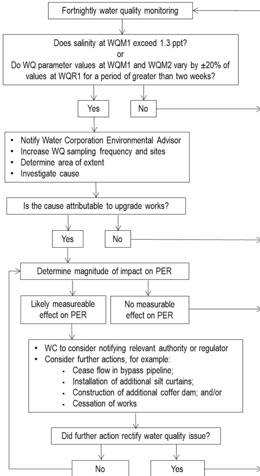
**Figure 4.** Water quality monitoring and management process for the Vasse River Diversion Dam Works Area.
