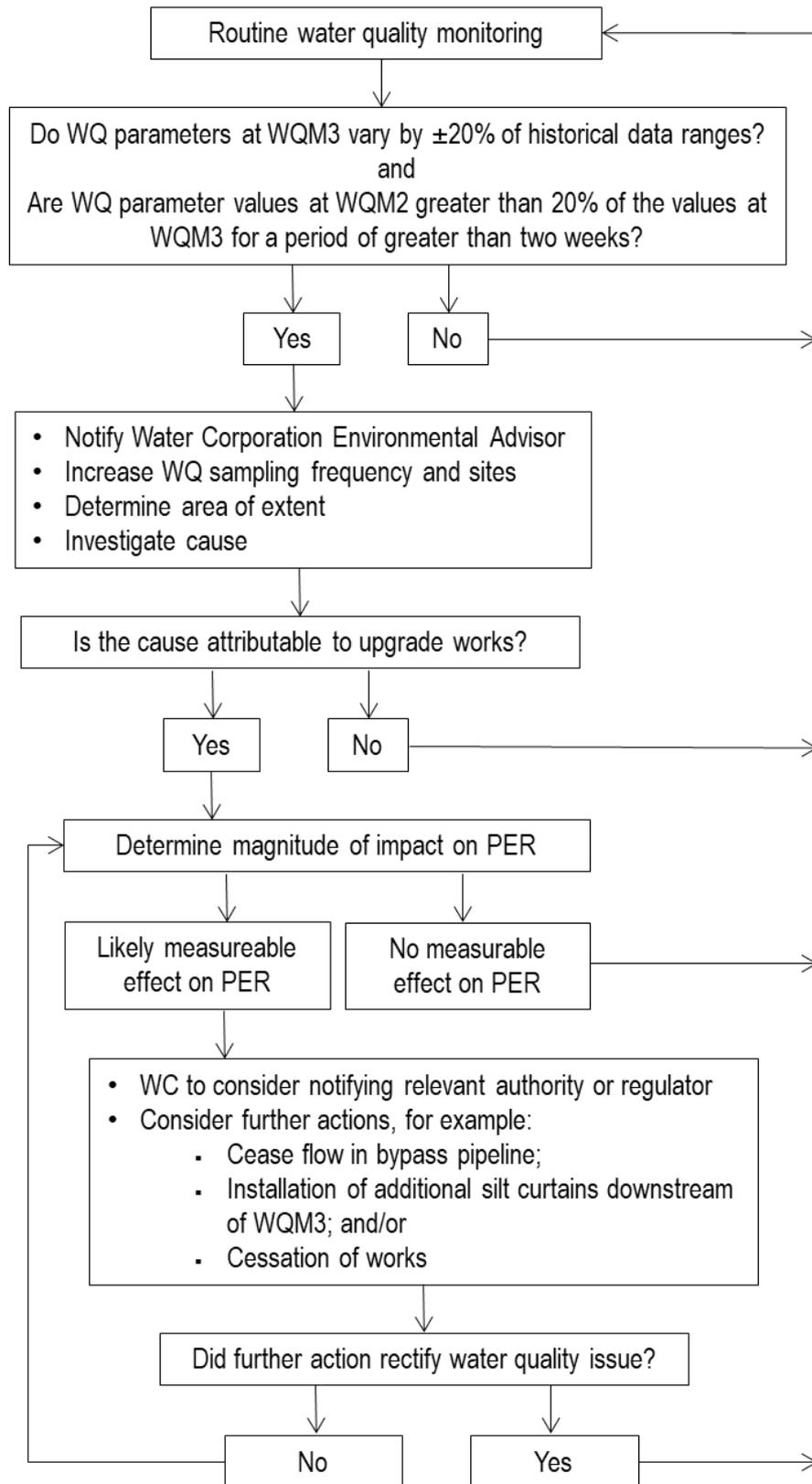
**Figure 5.** Water quality monitoring and management process for the Lower Vasse Diversion Drain Works Area.
