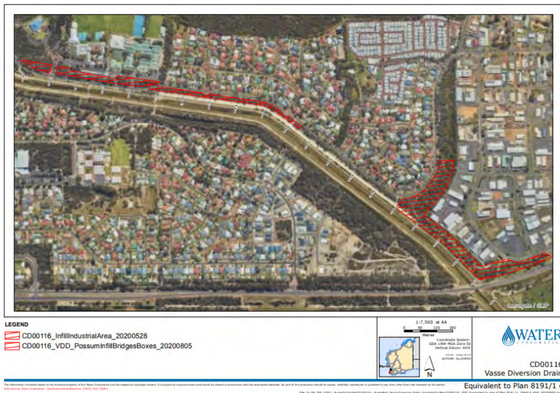
Figure 4. Map 8191/1c shows the areas in red crosshatch that require rope bridge and shelter installation.
