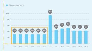
The water used by an evaporative air conditioner could appear similar to a leak in your online account. Ensure this is turned off when you are checking for leaks.
