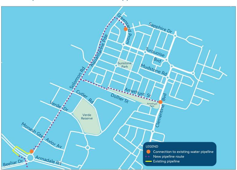
To cater for the growth forecast in the developing area of Jandakot and Treeby, Water Corporation is planning to install a new 2.6 km water pipeline. The location of the proposed work is shown on the map.
