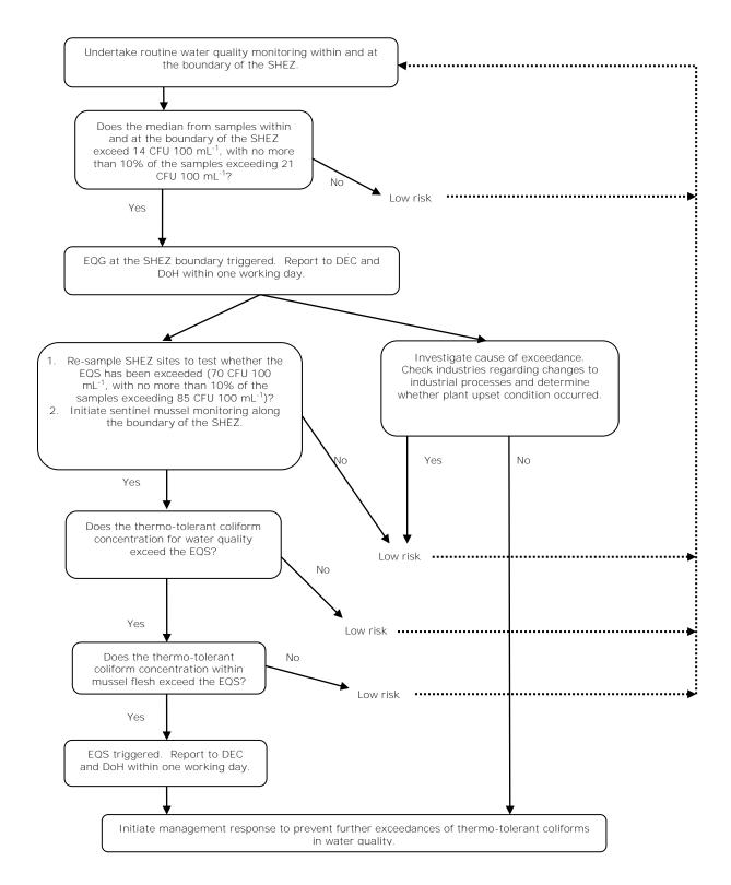
Figure B 5 Management response framework in the event of an exceedance of the EQC for thermo-tolerant coliforms in water and sentinel mussel tissues
