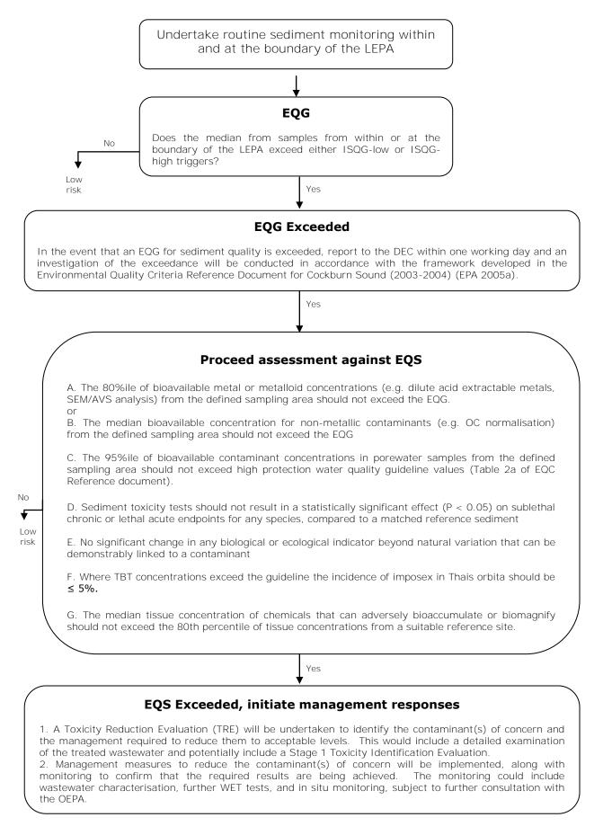
Figure B 4 Management response framework in the event of an exceedance of EQG (ISQG-low) triggers levels for sediment quality
