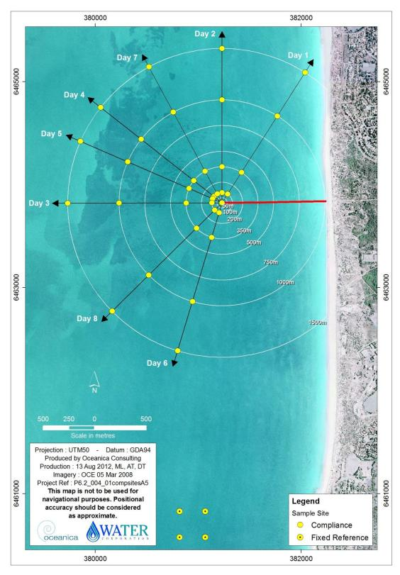
Figure 5.2 Conceptual diagram of the Compliance Monitoring program showing hypothetical compliance sites and their relative distances from the outlet diffuser
