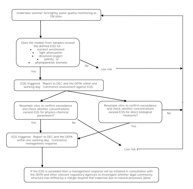
Figure B 3 Management response framework in the event of an exceedance of EQC triggers levels for receiving water quality: physico-chemical parameters and nutrient enrichment)
