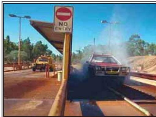
Figure 7.5 Vehicles are cleaned before entering uninfested areas
