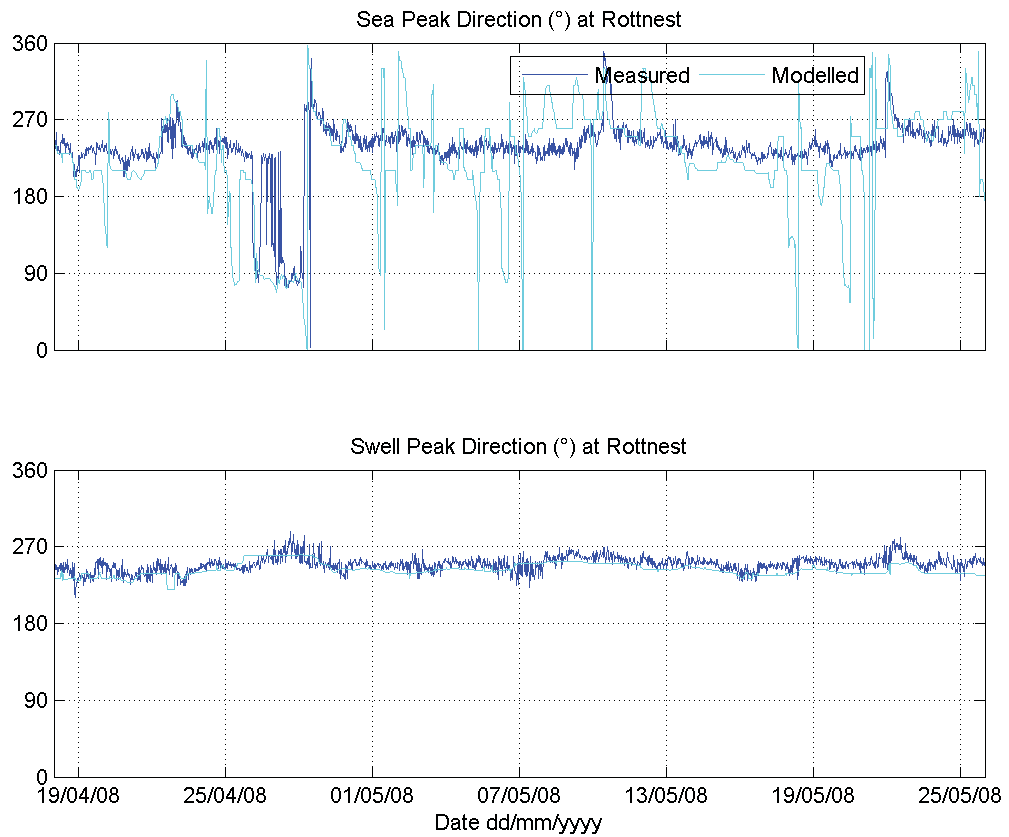
Figure 4-2: Time series of measured and modeled peak direction for sea and swell at the Rottnest buoy
