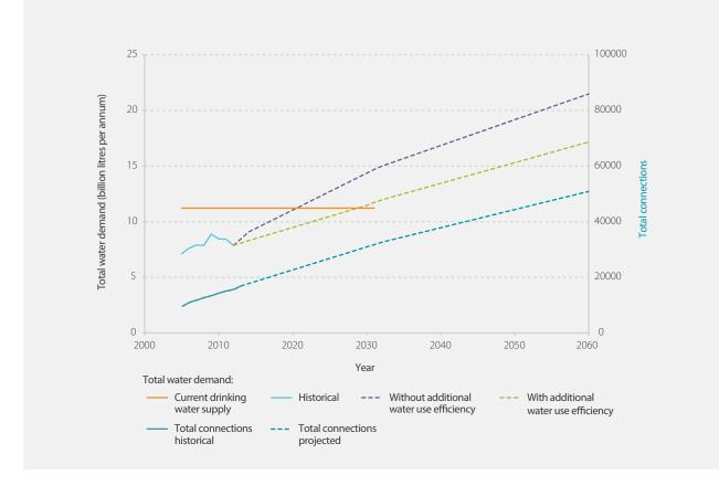
Figure 12 Projected water demand on the Swan Coastal Plain, with and without additional water use efficiency measures
