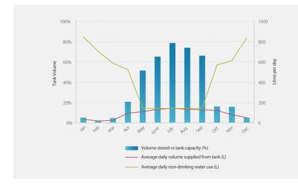
Figure 8 Australind rainwater tank capacity compared with average daily supply and use
