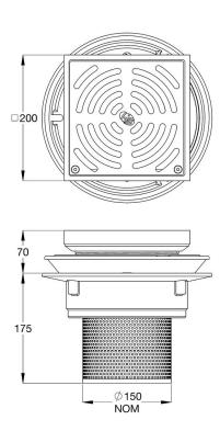
Cast stainless steel square floor drain assembly, threaded BSP, with stainless steel lock down Allen key screws, machined/linished surface, load rated to Class C, with grey enamel coated ductile iron multi-purpose body with reversible membrane collar with weep holes, stainless steel lock down screws, stainless steel adjustable removable strainer basket and secondary stainless steel fixed strainer basket.
