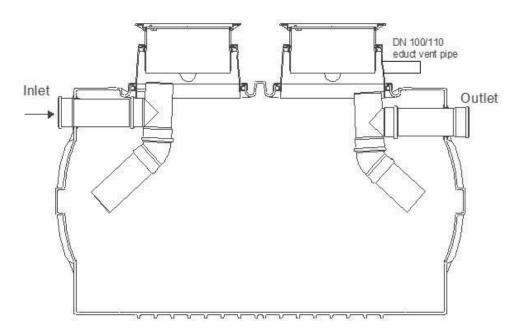
If the telescopic lid falls in front of the vent opening, please make sure to cut out the section that obstructs the venting as shown on the right.
