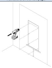
Use the 6 holes to secure the bracket to the wall.
