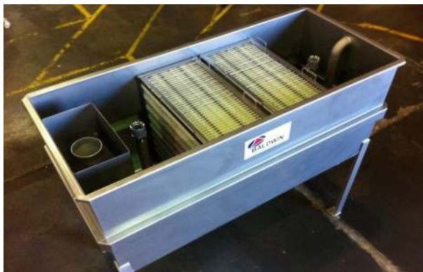
Correct Orientation of Plate Packs
