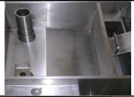
10. Install the stainless steel Breather Tube into the valve housing closest to the backside and turn it in the bayonet fitting to lock it into place.
