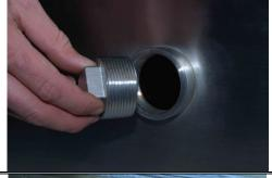
Screw the Threaded Plug into the unused heater boss on the backside of the unit. Use Teflon tape to ensure a good seal.
