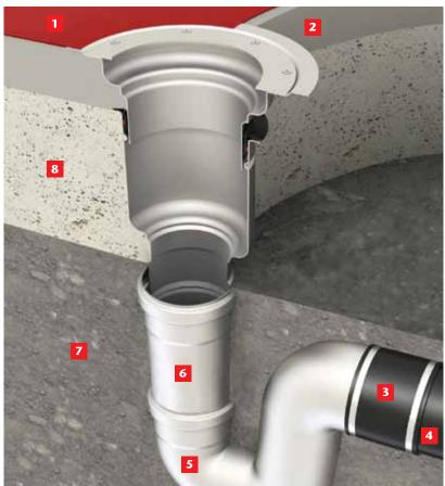
Adjustable height gully with internal FAT in suspended slab with a tile floor finish connecting into stainless pipe.
