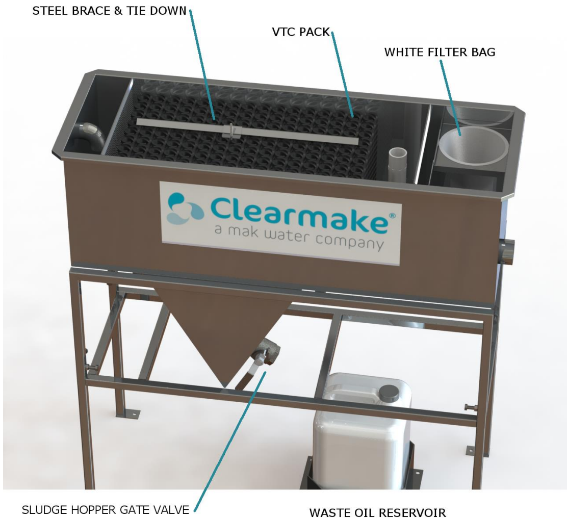
Figure 1 Separator Internal Parts
