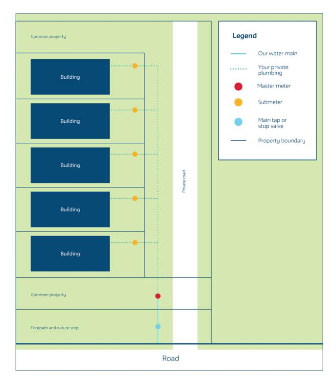
In this layout, the sub-meters must be located in front of the unit because they all come off the same private plumbing pipe.
