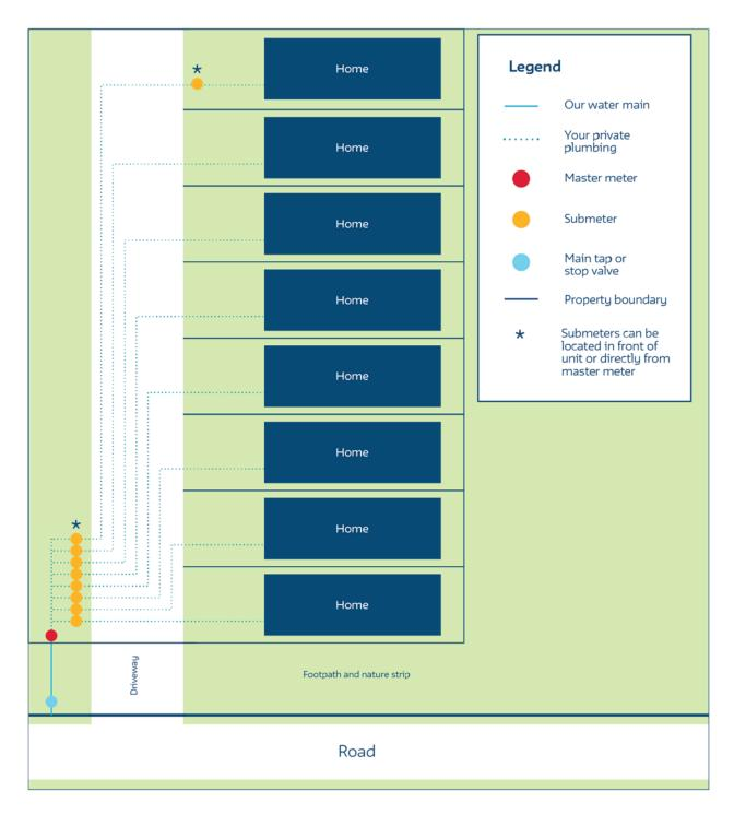
In this layout, the land is served with a master meter. Each unit is supplied off the master meter. Please note: the sub-meters can be located directly off the master meter or in front of the unit.
