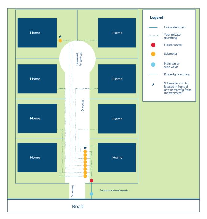
In this layout, the land is served with a master meter. Each unit is supplied off the master meter. Please note: the sub-meters can be located directly off the master meter or in front of the unit.
