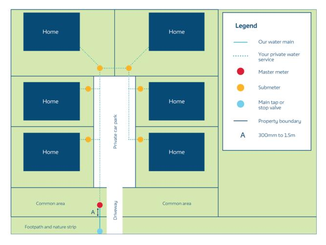
In this layout, the sub-meters must be located in front of the unit because they all come off the same private plumbing pipe.
