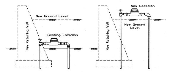
4. To **move your meter towards or away from house.**Regardless of the distance the meter is moved the charge is the same as moving your meter less than 500mm
