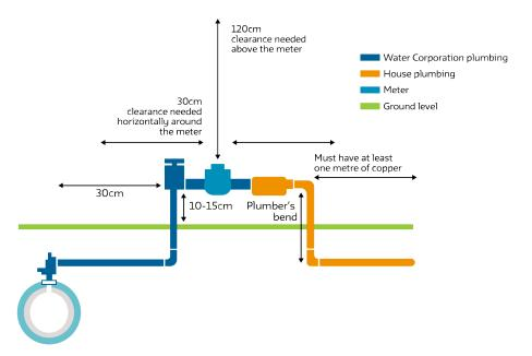
The clearances shown are required to facilitate meter reading and/or replacement when required. This is a requirement under the Water Services Regulations 2013
