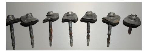
Photo 6 – Increasing "Localised Corrosion/Necking in Tek screw (Left to right).
