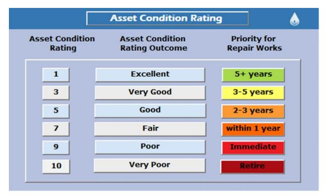
Figure 1 – Asset Condition Rating based on TDST model.
