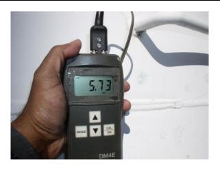
Photo 7 - Remaining Wall Thickness Measurement Gauge using UT gauge.
