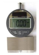
Photo 9 - ESR® Digital Pit Depth/Crack Gauge.
