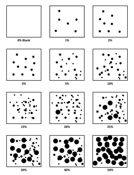
Figure 5 – Schematic representation of estimating rust percentages in 1 m2 area.
