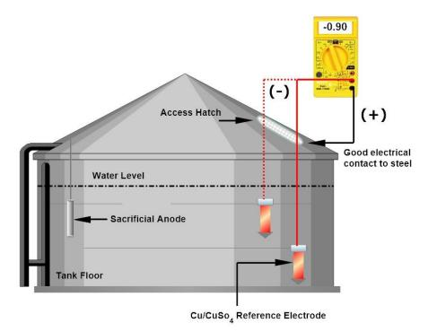
Figure 6 – CP potential measurement in the steel tank using portable Cu/CuSO<sub>4</sub> reference cell.
