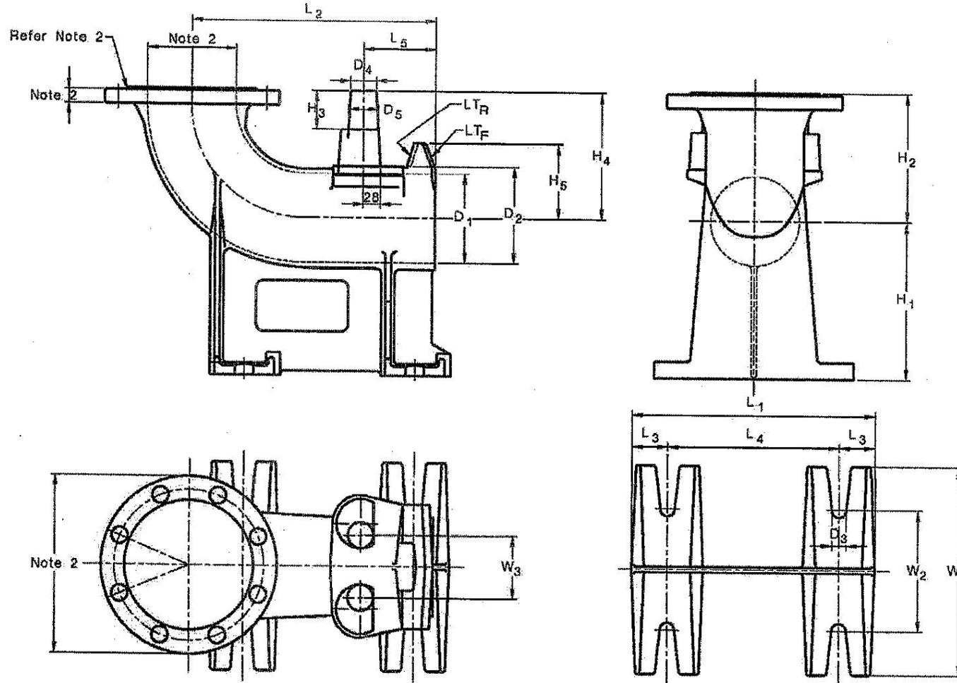
Fig 13.2 Standard Discharge Bend Detail Drawing - New 2008 Design - (Refer Table 13.1 for applicability and Dimensions)
