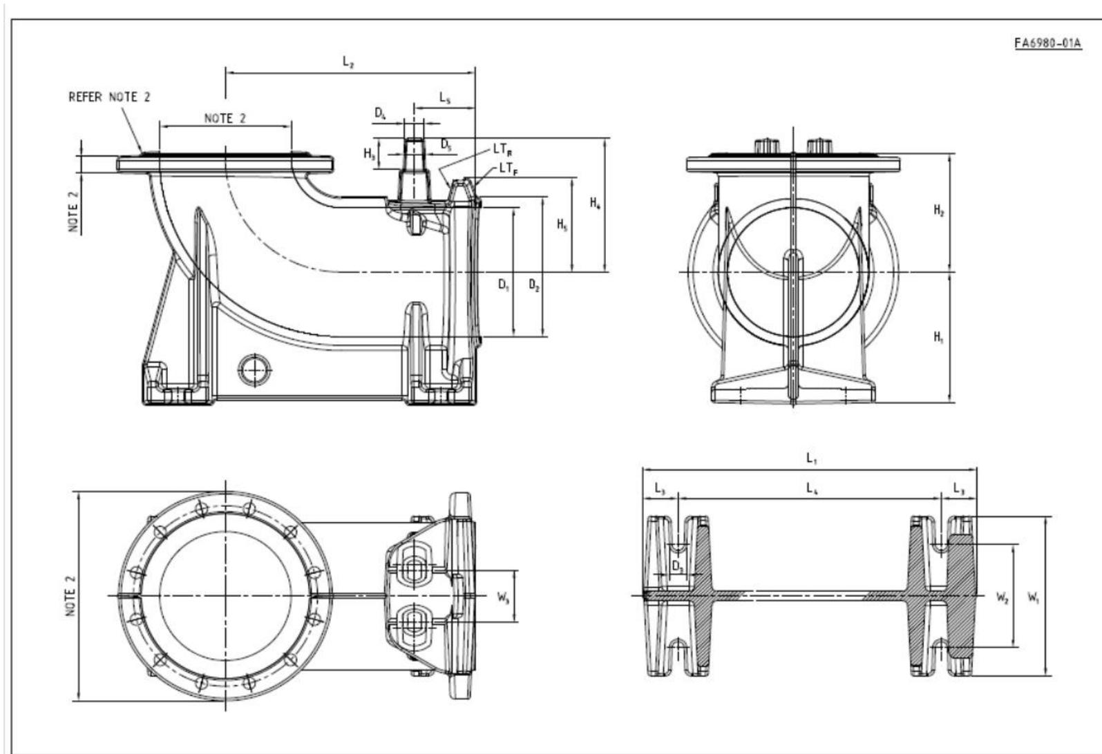
Table 13.1 Standard Discharge Bend (Original and New 2008 Design) Dimensions and Tolerances.
