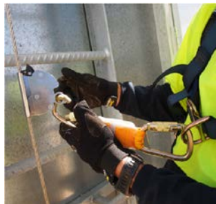
Figure 3-1 A cable grab on a ladder climbing system
