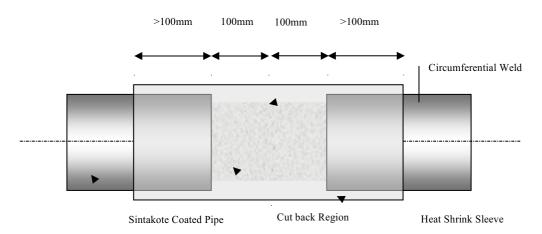
Figure 1 – Heat Shrink Sleeve Application.
