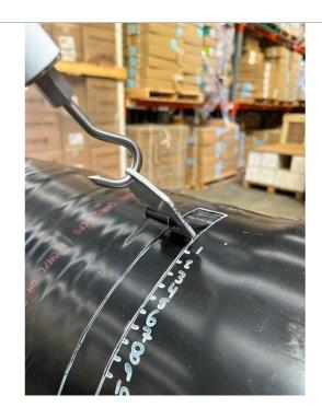
Peel Test set out in accordance with Appendix B of AS 4822;2018. Pass level is 5 kg.f (50 N) for a 25mm wide test sample.
