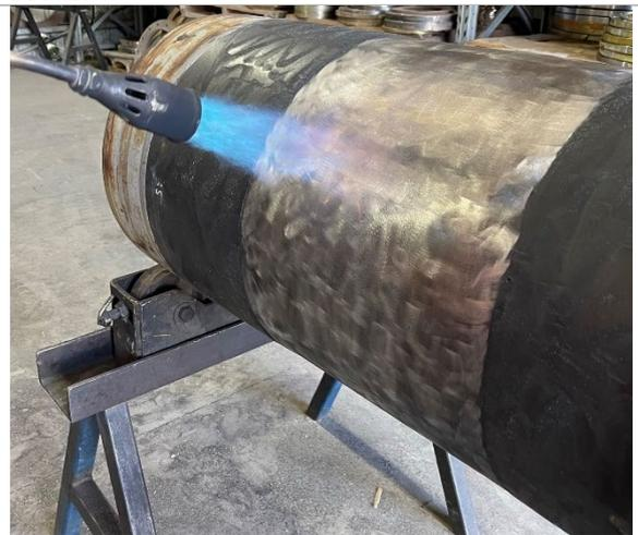
Pre-heat steel to 40-60°C using a propane torch with 50mm diameter burner head. For optimum HSS outcomes an auto ignition torch should be used, pictured below.
