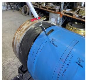
Peel Test set out in accordance with Appendix B of AS 4822;2018. Pass level is 5 kg.f (50 N) for a 25mm wide test sample.
