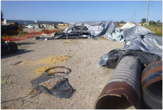
Figure 23 - Weathered asbestos coal tar coated pipe at Canning Vale Depot. Note the spiral wrap and coating colour weathered to light grey.
