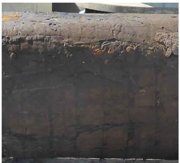
Figure 14 - Exhumed asbestos coal tar coated pipe originally installed in 1952. Close-up
