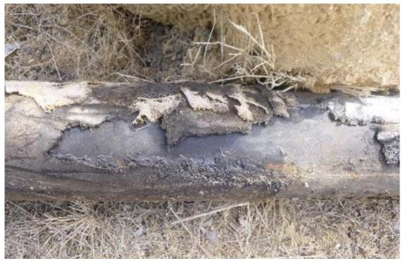
Figure 27 - Close-up of Greenmount pipe with a less common type of CTE coating consisting of an inner asbestos felt and outer protective layer (possibly fibreglass).
