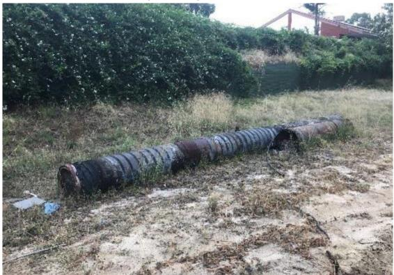
Figure 29 - Exhumed pipe at Lilac Place WWPS, Huntingdale. Note spiral wrap, coating colour weathered to grey and remnant whitewash.
