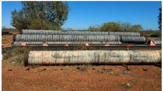
Figure 31 - Weathered asbestos coal tar coated pipes at South Hedland. Note the spiral bandage weathered to a light grey colour on the background pipes. The foreground CTE coated pipe has retained the protective whitewash over-coating.
