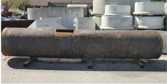
Figure 13 - Exhumed asbestos coal tar coated pipe originally installed in 1952. Note the coating deformation caused by soil stress and tree roots and the spiral wrap of the asbestos bandage.
