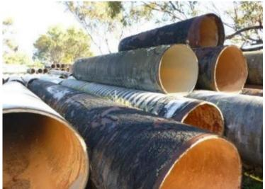
Figure 30 - Weathered coal tar coating at Kellerberrin Depot.
