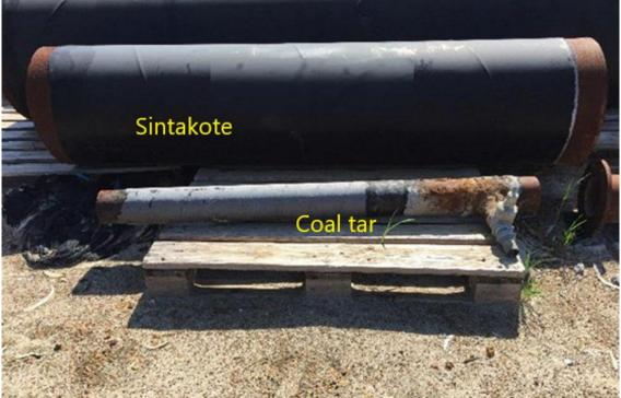
Figure 12 – Compare weathered fusion-bonded coated pipe (background) with weathered CTE-coated pipe (foreground).
