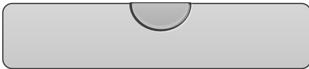
Figure 2 - Additional filler added to fill the pit. Do not bridge it.
