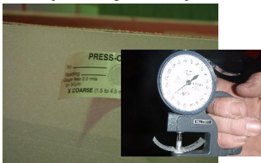
Figure 2: Blast Cleaned Surface Profile Measurement using TESTEX Tape
