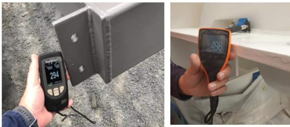
Figure 4: Measurement of DFT using electronic gauge.
