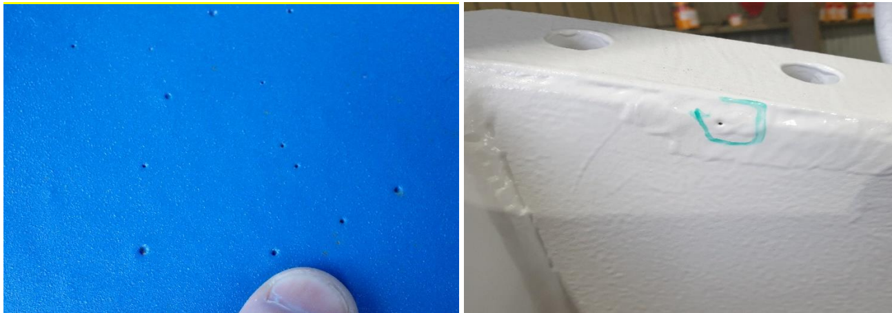
Figure 7: Pin holes detected during the spark testing
