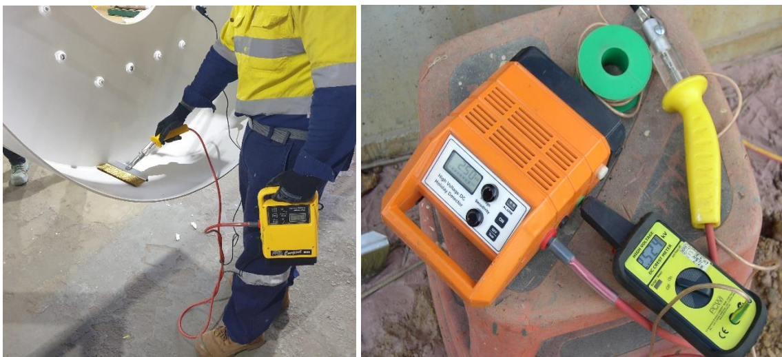
Figure 6: High Voltage Spark Tester calibrated using a Crest meter.
