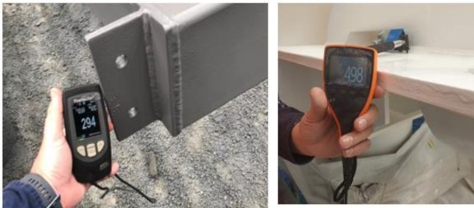
Figure 4: Measurement of DFT using electronic gauge.
