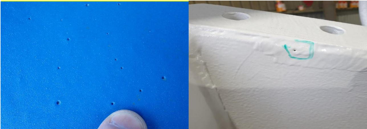
Figure 7: Pin holes detected during the spark testing
