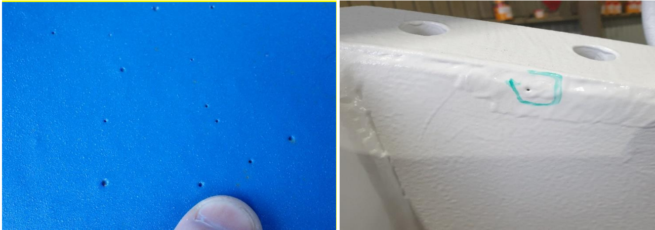
Figure 7: Pin holes detected during the spark testing
