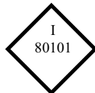
Figure 1: Example of an Interlock Symbol (on chlorine storage P&ID sheet 80.1)
