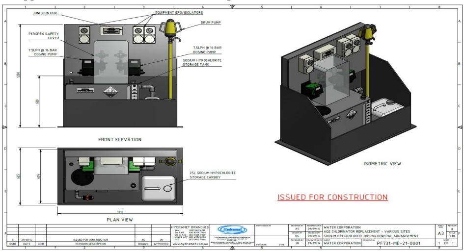
Figure 7-1: Dosing Pumps: Perspex box covers pressurised fittings on pump discharges – pipework passes through the panel itself. Pump and electrical connections not included within box
