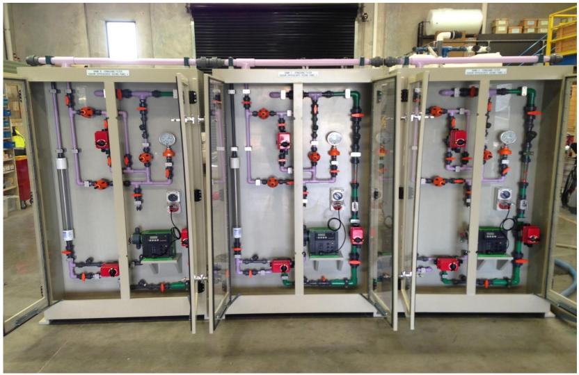
Figure 5-3: Large Enclosure – doesn't include pump and electrical cutouts but does illustrate space provision for maintenance activities
