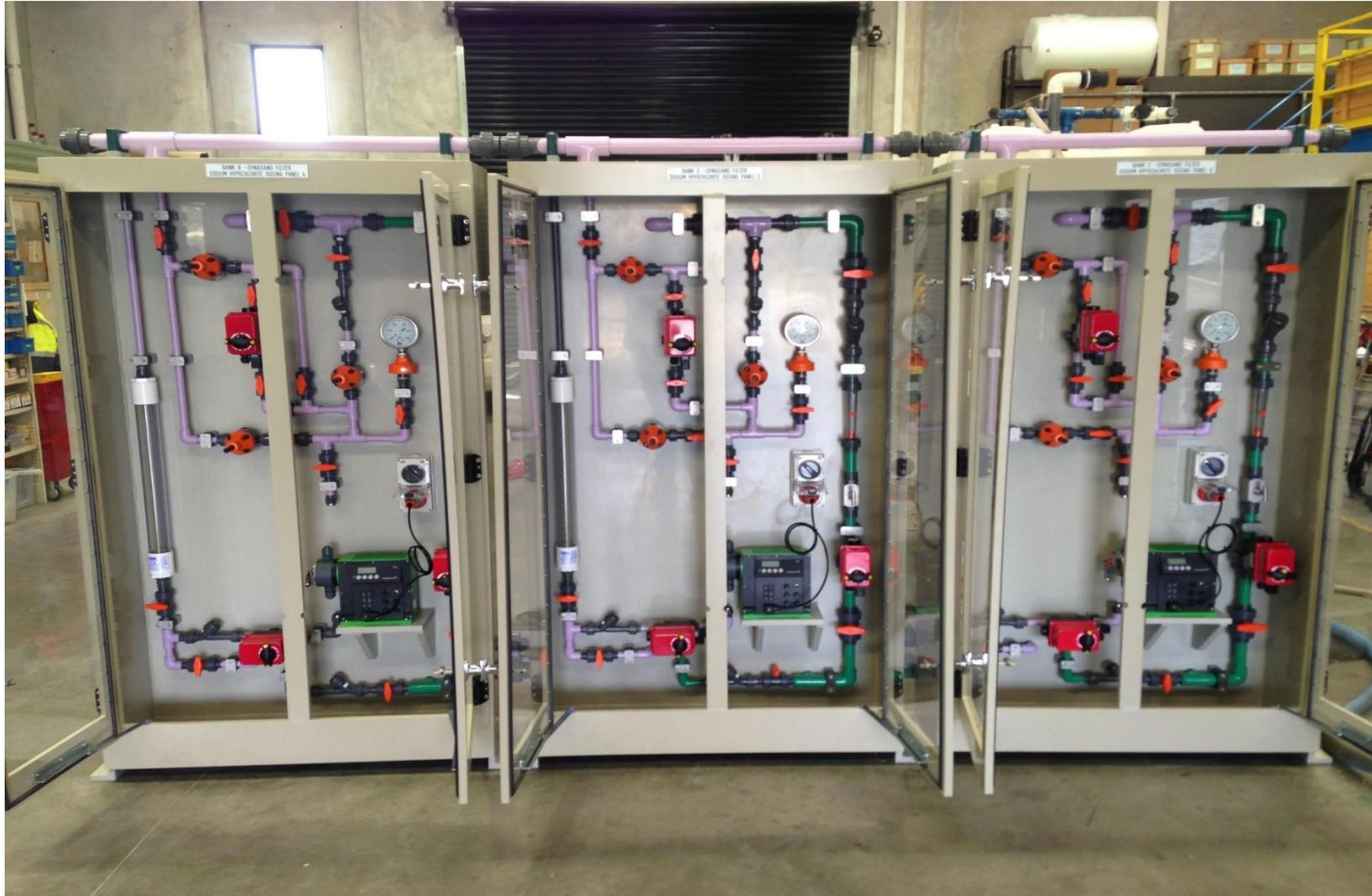
**Figure 5-3: Large Enclosure – doesn't include pump and electrical cutouts but does illustrate space provision for maintenance activities**
