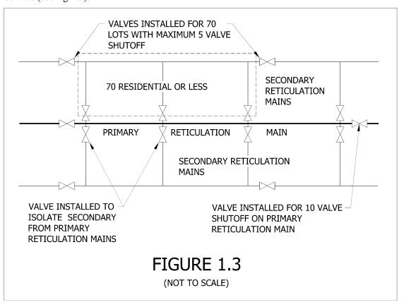
A primary reticulation main supplies water to a number of secondary reticulation mains. The primary reticulation main is normally a 200mm or 250mm diameter main supplying 150mm and 100mm secondary reticulation mains. Generally the primary reticulation main is:
