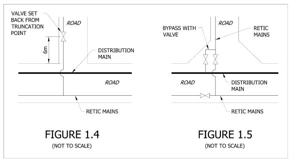
Intersecting mains shall be arranged in a configuration as typically shown on the drawings of this Standard.
