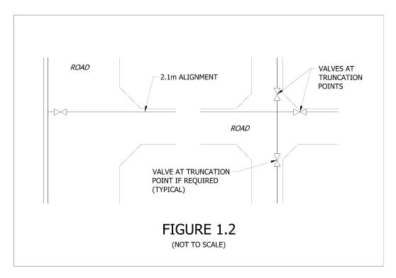
• where street corners have truncations larger than the standard, such as at an intersection that incorporates a major roundabout with extensive landscaping, the Corporation may require the mains to follow the boundaries on the 2.1m standard alignment.
