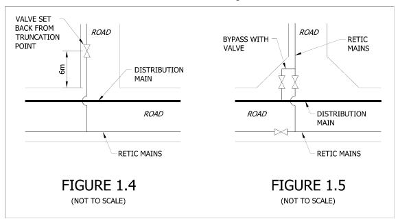
Intersecting mains shall be arranged in a configuration as typically shown on the drawings of this Standard.
