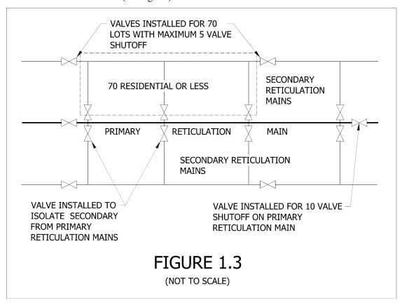
A primary reticulation main supplies water to a number of secondary reticulation mains. The primary reticulation main is normally a 200mm or 250mm diameter main supplying 150mm and 100mm secondary reticulation mains. Generally the primary reticulation main is:
