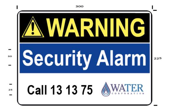
This **Security Warning** sign is in landscape format with a standard warning title block with yellow text on a black background at the top of the sign. The middle text block shall be white text on a dark blue background. The base background of the sign is white with black text and the standard Water Corporation logo on the bottom section. Material: Metal or Vinyl – 300 (W) x 225 (H) with the other dimensions as indicated.
