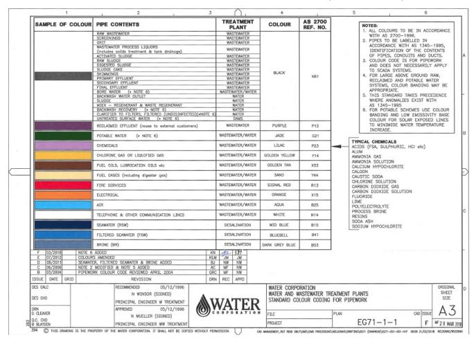
The above Water Corporation **Colour Coding** standard complies with "AS 2700:2011" and "AS 1345:1995" for pipework located at water and wastewater plants/facilities.
