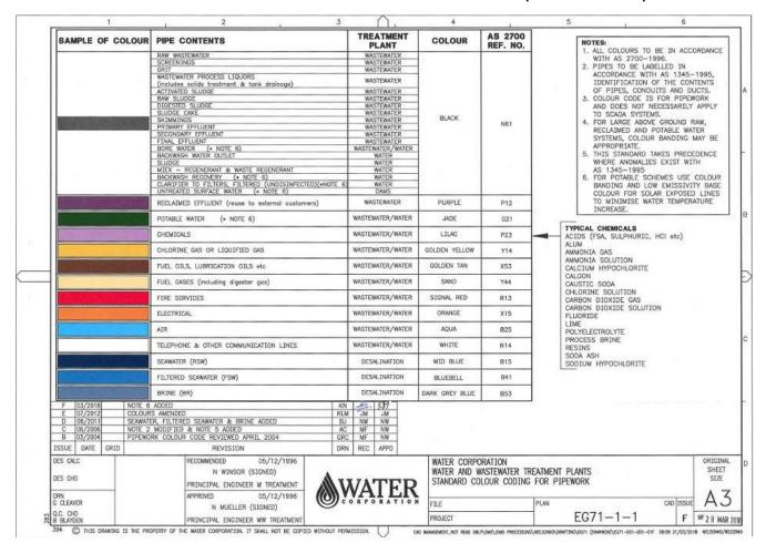
The above Water Corporation **Colour Coding** standard complies with "AS 2700:2011" and "AS 1345:1995" for pipework located at water and wastewater plants/facilities.
