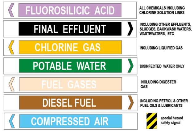
WATER CORPORATION, WATER & WASTEWATER STANDARD COLOUR CODING FOR PIPEWORK: DWG No. EG71-1-1
