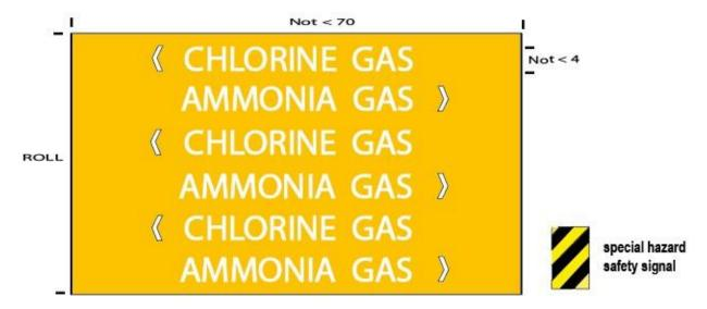
This **Identification Marker** is for pipe or tubing **less than 40mm** in diameter as per AS 1345 - 1995.
