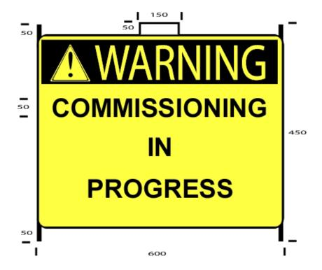
This **Hazard Warning** sign is in landscape format with a standard warning symbol as per AS1319. The other text shall be black on a yellow background. Material: Metal – 600 (W) x 450 (H) with the other dimensions as indicated Design: Sign attached to a reversible 'A' frame with carry handle.
