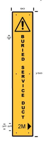
This **Hazard Warning** sign is a vertical sign with a standard warning symbol and black 25mm text on a yellow background (note that the arrow(s) may be placed on the right, left or both sides).
