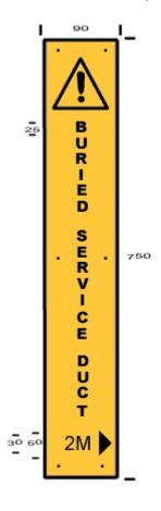
This **Hazard Warning** sign is a vertical sign with a standard warning symbol and black 25mm text on a yellow background.
