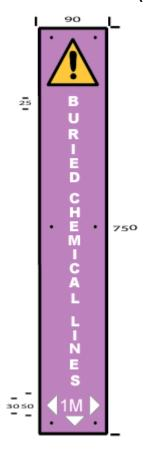
This **Hazard Warning** sign is a vertical sign with a standard warning symbol and white 25mm text on a lilac background (note that the arrow(s) may be placed on the right, left or both sides). Material: Metal  $-90 \text{ (W)} \times 750 \text{ (H)}$ .
