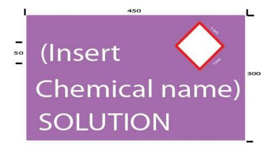
This **Hazardous Chemicals** sign has white text on a lilac background. Material: Metal or Vinyl (note that the dimensions are dependent on the size of the tank, but the text shall be no less than 50mm in size).
