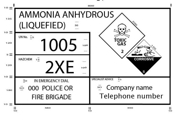
This **Transport Emergency Information Panel (EIP)** has black text on a white background with the specified division and subsidiary hazard labels as per the Australian Code for the Transport of Dangerous Goods by Road & Rail (ADG Code). Material: Metal or Vinyl – 800 (W) x 600 (H) with the other dimensions as indicated.
